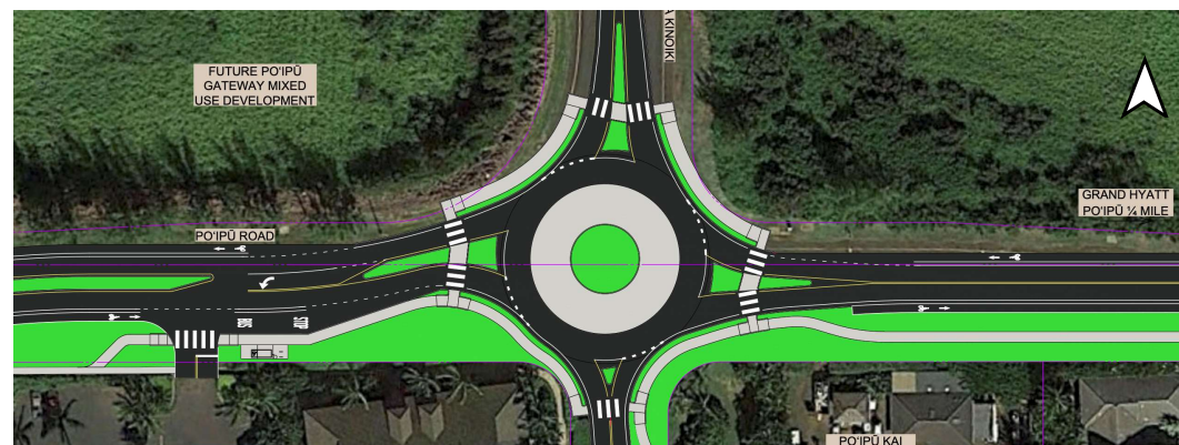
FIGURE 10: PO'IPŪ ROAD CONCEPT PLAN AT THE INTERSECTION WITH ALA KINOIKI AND PE'E ROAD
