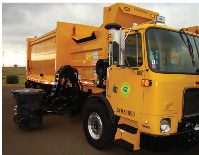
Automated truck and cart
