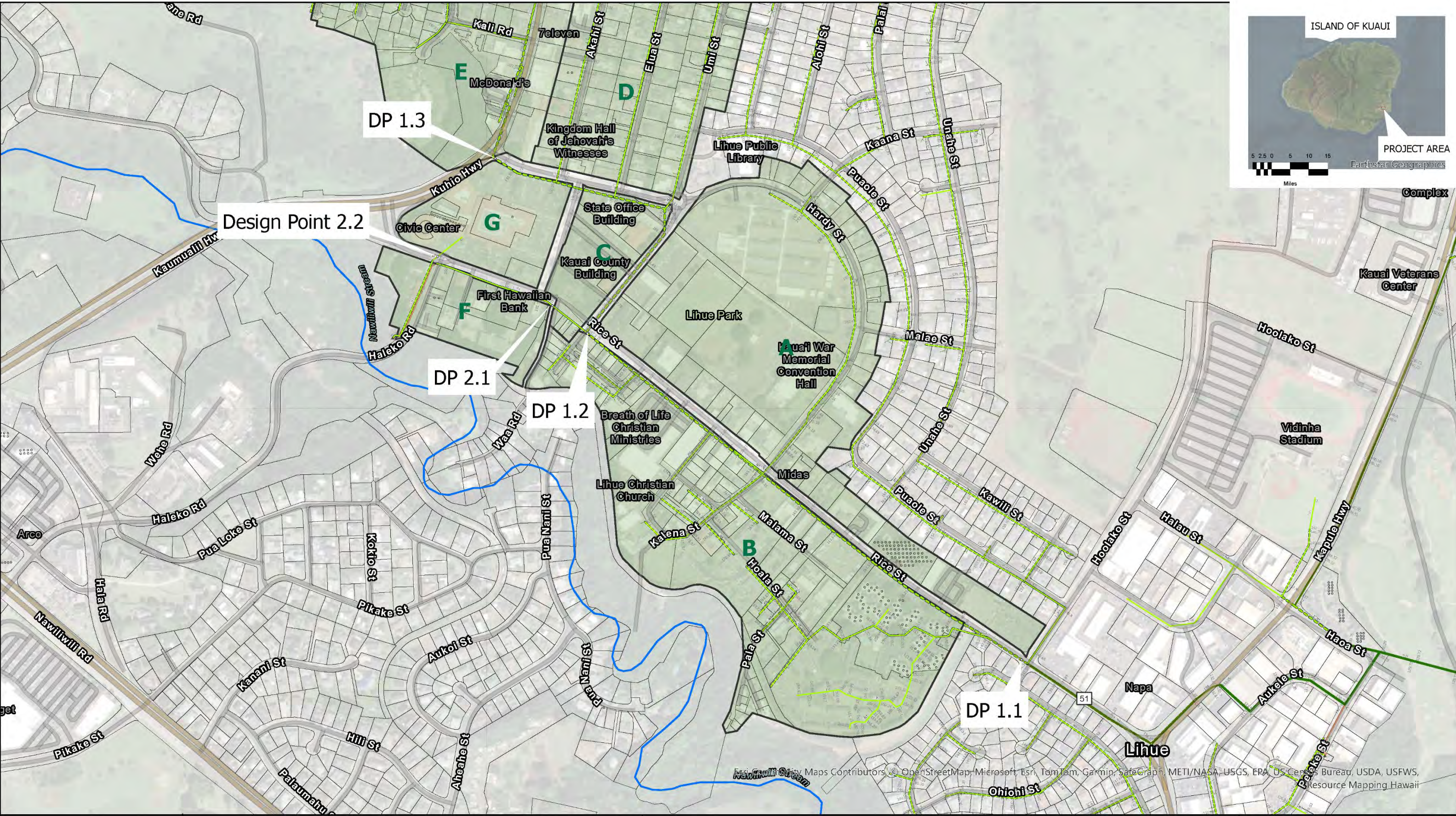
References: - Sewer & water line data received from the County of Kauai on 11/14/2023 - Contour data retrieved from the USGS National Map on 02/07/2024 - Streams data retrieved from the Hawaii Geoportal on 02/21/2024 Figure 1. Existing Sewer Lines and Design Points for Existing Flow Analysis
