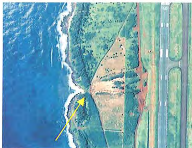
Photo A4 - Wash out area where a new culvert pipe and safety railings will be required in order to accommodate the path.
