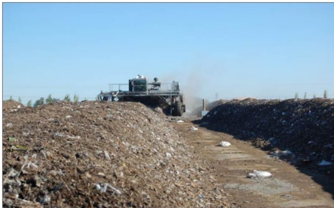
Figure 8: Example of a Windrow Aerobic Composting Facility
